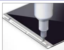
Conductive Ag paste dispensing on touch panels
