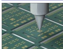
Ag paste dispensing for die bonding
