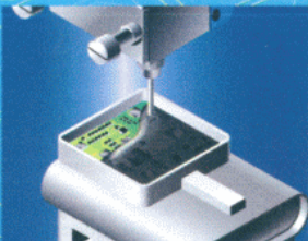
Gel filling in sensor parts
